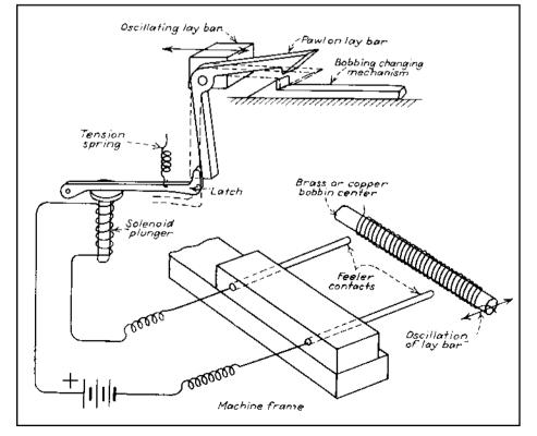
**Fig. 3** Bobbin changer. When a bobbin is empty, the feeders contact the metal bobbin center, completing the circuit through a solenoid which pulls a latch. That causes the bobbin-changing mechanism to operator and put a new bobbin in the shuttle. As long as the solenoid remains deenergized, the pawl on the lay bar is raised clear of the hook on the bobbin-changing mechanism.
