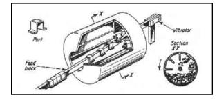
A barrel hopper is useful if parts lend to become entangled. The parts drop free of the rotating-barrel sides. By chance selection, some of them fall onto the vibrating rack and are fed out of the barrel. The parts should be stiff enough to resist excessive bending because the tumbling action can subject them to relatively severe loads. The tumbling can help to remove sharp burrs.
