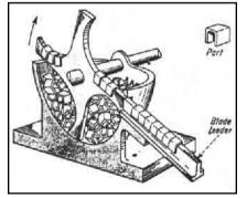
Rotary centerblades catch small Ushaped parts effectively if their legs are not too long. The parts must also be resilient enough to resist permanent set from displacement forces as the blades cut through a pile of parts. The feed is usual continuous.
