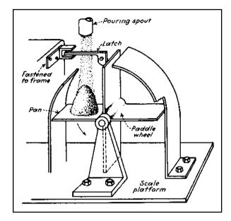
**Fig. 22** When the predetermined weight of material has been poured on the pan, the movement of the scale beam pushes the latch out of engagement. This allows the paddle wheel to rotate and dump the load. The scale beam drops, thereby returning the latch to the holding position and stopping the wheel when the next vane hits the latch.
