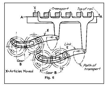
**Fig. 6** An arrangement of interconnected gears with equal diameters that will impart a transport motion to a mechanism. The gear and link mechanism imparts both the forward motion and the raising and lowering motions. The gear shafts are supported in the frame of the machine.
