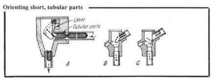
Here's a common problem; Parts arrive in either open-end or closed-end first; you need a device that will orient all the parts so they feed out facing the same way. In Fig. A. when a part comes in open-end first, it is pivoted by the swinging lever so that the open end is up. When it comes in closed-end first, the part brushes away the lever to flip over headfirst. Fig. B and C show a simpler arrangement with pin in place of lever.
