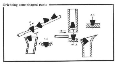
Regardless of which end of the cone faces forward as the cones slide down the cylindrical rods, the fact that both rods rotate in opposite directions causes the cones to assume the position shown in section A-A (above). When the cones reach the thinned-down section of the rods, they fall down into the chute, as illustrated.
