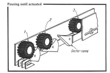
Each gear in this device is held up by a pivotable cam sector until the gear ahead of it moves forward. Thus, gear 3, rolling down the chute, kicks down its sector cam but is held up by the previous cam. When gear 1 is picked off (either manually, or mechanically), its sector cam pivots clockwise because of its own weight. This permits gear 2 to move into place of gear 1—and frees cam 2 to pivot clockwise. Thus, all gears in the row move forward one station.
