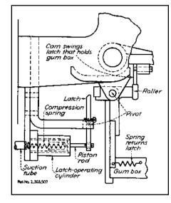
**Fig. 2** The gumming of the suction picker and label carrier when the label is not picked up by the suction is prevented by insufficient suction on a latch-operating cylinder, caused by open suction holes on the picker. When a latch-operating cylinder does not operate, the gum box holding latch returns to its holding position after cyclic removal by the cam and roller, thus preventing the gum box and rolls from rocking to make contact with the picker face.
