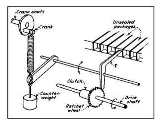
**Fig. 24** some package-loading machines have provisions to stop the machine if a package passes the loading station without receiving an insert. Pawl finger F has a rocking motion imparted by the crankshaft, timed so that it enters the unsealed packages and is stopped against the contents. If the box is not filled, the finger enters a long distance. The pawl end at the bottom engages and holds a ratchet wheel on the driving clutch which disengages the machine-driving shaft.
