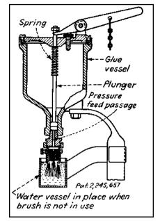
Fig. 13 A brush applicator is fed through passages between bristle tufts by a spring-operated plunger.
