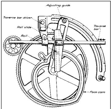
**Fig. 5** A roll that rides in a heart-shaped cam groove engages a slot in a traverse bar driver which is attached to the traverse bar. Maximum traverse is obtained when the adjusting guide is perpendicular to the driver. As the angle between the guide and driver is decreased, traverse decreases proportionately. Inertia effects limit this mechanism to slow speeds.
