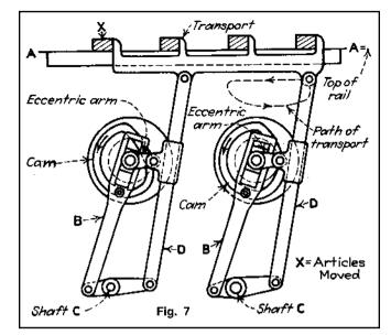
**Fig. 7** In this transport mechanism, the forward an return strokes are accomplished by the eccentric arms, while the vertical motion is performed by the cams.
