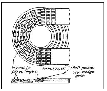
A rotary conveyor transfers articles from one belt conveyor to another without disturbing their relative positions.
