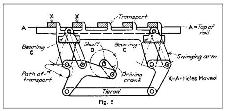
**Fig. 5** This is another form of transport mechanism based on a link motion. The bearings C are supported by the frame as is the driving shaft D.
