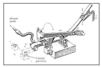
**Feeding special-shaped parts.** Parts of such special shapes as shown are removed, one by one, in a given direction, and are then moved individually into the corresponding indents on transfer platforms.
