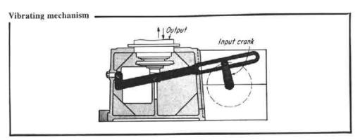
As the input crank rotates, the slotted link, which is fastened to the frame with an intermediate link, oscillates to vibrate the output table up and down.
