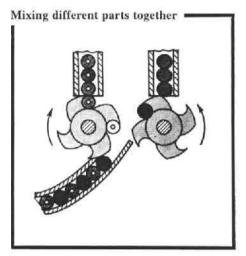
Two counter rotating wheels form a simple device for alternating the feed of two different workpieces.
