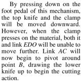
Parallel cutter mechanisms
