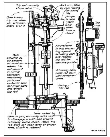
Fig. 6 A nozzle on the packaging machine does not open when the container is improperly positioned.
