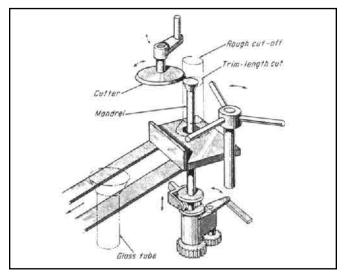
**Cutoff and transfer devices for glass tubes.** The upper part of a rotating glass tube is held by a chuck (not shown). When the cutter cuts the tube to a given length, the mandrel comes down and a spring member (not shown) drops the tube on the chute.
