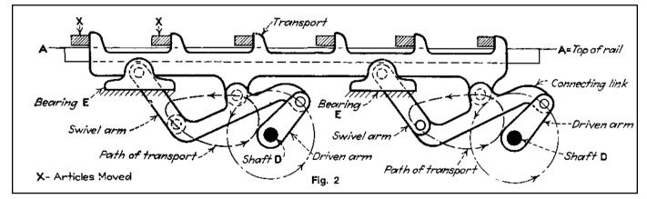
**Fig. 2** Here is a simple form of linkage that imparts a somewhat "egg-shaped" motion to the transport. The forward stroke is almost a straight line. The transport is carried on the connecting links. As in the design of Fig. 1, the shafts *D* are driven in unison and are supported in the frame of the machine. Bearings *E* are also supported by the frame of the machine and the rail *A*-*A* is fixed.
