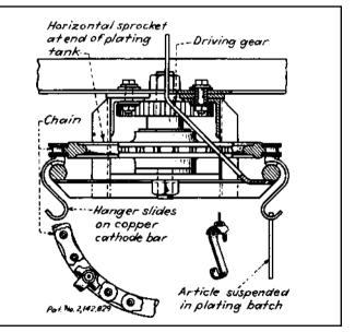
Hooks on a chain-driven conveyor move articles through a plating bath.
