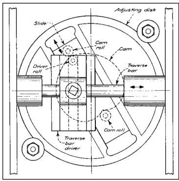
**Fig. 6** The two cam rolls that engage this heart-shaped cam are attached to the slide. The slide has a driver roll that engages a slot in the traverse bar driver. Maximum traverse (to the capacity of the cam) occurs when the adjusting disk is set so the slide is parallel to the traverse bar. As the angle between the traverse bar and slide increases, traverse decreases. At 90° traverse is zero.
