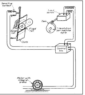
**Fig. 6** This automatic stop for a folder or yarder machine always stops the machine in the same position when a seam in the cloth passes between the rolls. A seam passing between the rolls causes the swivel-mounted roll to lift slightly. This motion closes contacts in a sensitive switch that opens a relay in the control box. The next time the cam closes the limit switch, the power of the motor with the integral magnetic brake is shut off. The brake always stops the machine in the same place.
