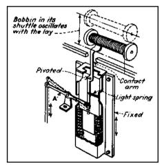
**Fig. 20** A diagram of a mechanism that causes a bobbin changer to operate. If the contact arm does not slip on the bobbin, lever A will rotate to the position shown. But if contact with the bobbin center slips, when the bobbin is empty, lever A will not rotate to the position indicated by the dashed line. This will cause the bobbin changer to operate.
