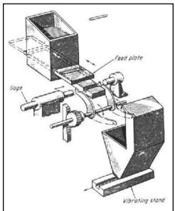
Horizontal feed for fixed-length rods. Single rods of a given length are brought from the hopper to the slot of a fixed plate by a moving plate. After being gauged in the notched portion of the fixed plate, each rod is moved to the chute by means of a lever, and is removed from the chute by a vibrating table.
