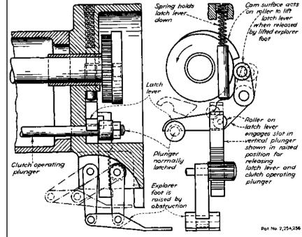
**Fig. 7** An obstruction under the explorer foot of a wire-stitching machine raises a vertical plunger which releases a latch lever. A rotary cam then raises a lever that retains the clutch-operating plunger.
