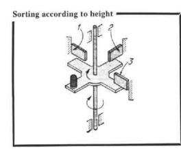
Workpieces of varying heights are placed on this slowly rotating crossplatform. Bars 1, 2, and 3 have been set at decreasing heights beginning with the highest bar (bar 1), down to the lowest bar (bar 3). The workpiece is therefore knocked off the platform at either station 1, 2, or 3, depending on its height.
