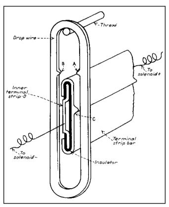
**Fig. 5** Electric stop for a loom. When a thread breaks or slackens, the drop wire falls and contact A rides on contact C. The drop wire, supported off-center, swings so that contact B is pulled against the inner terminal strip D, completing the solenoid circuit.
