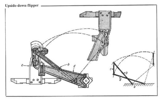
This is a four-bar linkage (links a, b, c, d) in which the part to be turned over is coupler c of the linkage. For the proportions shown, the 180° rotation of link c is accomplished during the 90° rotation of the input link.
