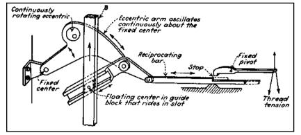
**Fig. 19** When thread breaks, the stop drops and intercepts the reciprocating bar. On the next counter-clockwise oscillation of the eccentric arm, the bar *B* is raised. A feature of this design is that it permits the arm *B* to move up or down independently for a limited distance.
