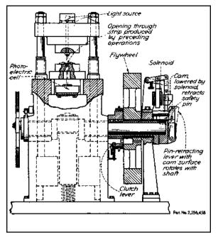
**Fig. 4** A high-speed press is stopped when a metal strip advances improperly. A hole punched in the strip fails to match while the opening in the die block to permit a light beam to pass. When the light beam to the photoelectric cell is blocked, the solenoid which withdraws the clutch pin is activated.
