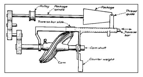
**Fig. 1** A package is mounted on a belt-driven shaft on this precision winding mechanism. A camshaft imparts reciprocating motion to a traverse bar with a cam roll that runs in a cam groove. Gears determine the speed ratio between the cam and package. A thread guide is attached to the traverse bar, and a counterweight keeps the thread guide against the package.
