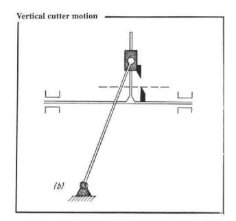
The top knife in this arrangement remains parallel to the bottom knife at all times during cutting to provide a true scissor-like action, but friction in the sliding member can limit the cutting force.
