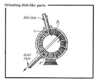
A part with its open-end facing to the right (part 1) falls on a matching projection as the indexing wheel begins to rotate clockwise. The projection retains the part for 230° to point A where it falls away from the projection to slide down the outlet chute, open-end up. An incoming part facing the other way (2) is not retained by the projection, hence it slides *through* the indexing wheel so that it too, passes through the outlet with its open-end up.
