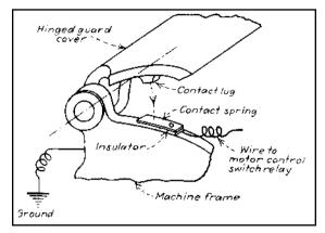
**Fig. 1** A safety mechanism on some machines stops the motor when a guard cover is lifted. The circuit is complete only when the cover is down. In that position a contact lug establishes a metal-to-metal connection with the contact spring, completing the relay circuit.
