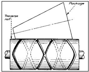
**Fig. 2** A package is friction-driven from a traverse roll. Yarn is drawn from the supply source by traverse roll and is transferred to a package from the continuous groove in the roll. Different winds are obtained by varying the grooved path.
