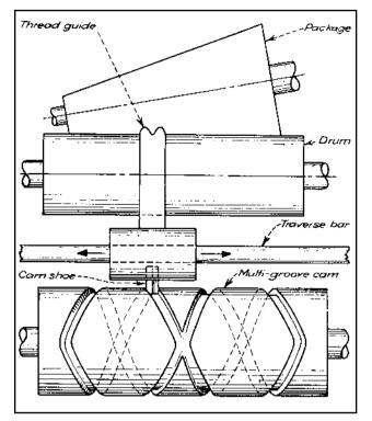
**Fig. 4** A drum drives the package by friction. A pointed cam shoe, which pivots in the bottom side of the thread guide assembly, rides in cam grooves and produces a reciprocating motion of the thread guide assembly on the traverse bar. Plastic cams have proved to be satisfactory even with fast traverse speeds. Interchangeable cams permit a wide variety of winding methods.
