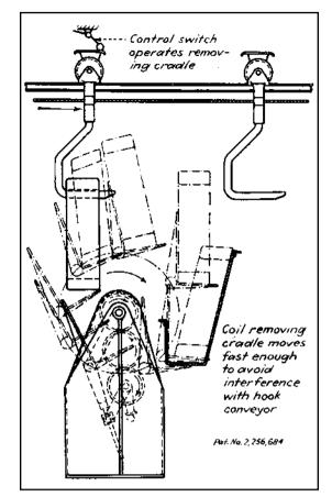
Hooks on a cable-driven conveyor and an automatic cradle for removing coils.
