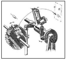
Feeding electronic components. Capacitors, for example, can be delivered by a pair of intermittently rotating gearlike disks with notched circumferences. Then a pick-up arm lifts the capacitor and it is carried to the required position by the action of a cam and follower.
