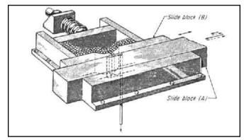
**Vertical feed for wires.** Wires of fixed length are stacked vertically, as illustrated. They are removed, one by one, as blocks A and B are slid by a cam and lever (not shown) while the wires are pressed into the hopper by a spring.
