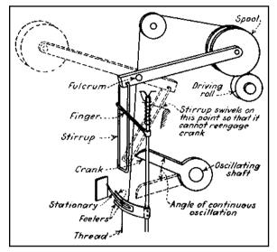
**Fig. 17** A mechanism on a spooler. When a thread breaks, the feelers are released and the spiral spring causes the spindle with finger to rotate. The finger throws the stirrup into the path of the oscillating crank, which on its downward stroke throws the spool into the position shown dotted. The stirrup is then thrown out of the path of the oscillating crank.
