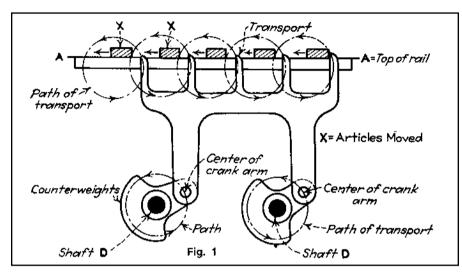
**Fig. 1** In this design a rotary action is used. The shafts *D* rotate in unison and also support the main moving member. The shafts are carried in the frame of the machine and can be connected by either a link, a chain and sprocket, or by an intermediate idler gear between two equal gears keyed on the shafts. The rail *A*-*A* is fixed rigidly on the machine. A pressure or friction plate can hold the material against the top of the rail and prevent any movement during the period of rest.
