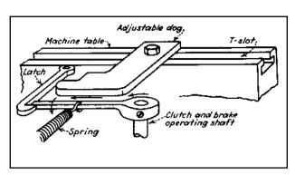
**Fig. 21** A simple stop mechanism for limiting the stroke of a reciprocating machine member. Arrows indicate the direction of movements.
