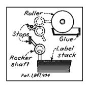
Fig. 16 A rocker shaft on a rack, which is moved vertically by a sector gear, carries glue on a contact bar from the roll to the label stack.
