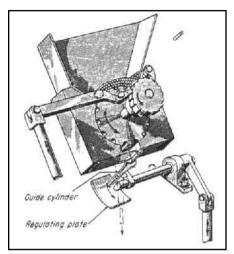
**Gravity feed for rods.** Single rods of a given length are transferred from the hopper to the lower guide cylinder by means of an intermittently rotating disk with a notched circumference. The guide cylinder, moved by a lever, delivers the rod when the outlet moves free of the regulating plate.
