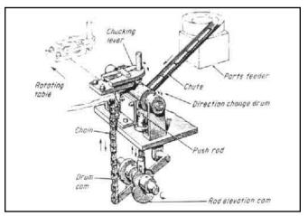
**Vertical feed for rods.** Rods supplied from the parts-feeder are fed vertically by a direction drum and a pushing bar. The rod is then drawn away by a chucking lever.
