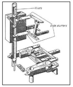
**Feeding headed rivets.** Headed rivets, correctly oriented, are supplied from a partsfeeder in a given direction. They are dropped, one by one, by the relative movement of a pair of slide shutters. Then the rivet falls through a guide cylinder to a clamp. Clamp pairs drop two rivets into corresponding holes.
