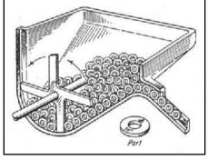
A paddle wheel is effective for feeding diskshaped parts if they are stable enough. Thin, weak parts would bend and jam. Avoid these designs, if possible—Especially if automatic assembly methods will be employed.
