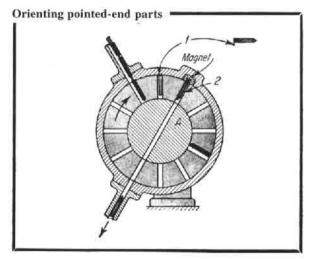
The important point here is that the built-in magnet cannot hold on to a part as it passes by if the part has its pointed end facing the magnet. Such a correctly oriented part (part 1) will fall through the chute as the wheel indexes to a stop. An incorrectly oriented part (part 2) is briefly held by the magnet until the indexing wheel continues on past the magnet position. The wheel and the core with the slot must be made from some nonmagnetic material.
