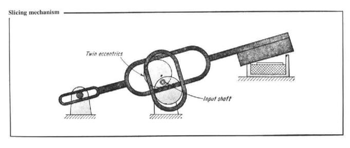
Slicing motion is obtained from the synchronized effort of two eccentric disks. The two looped rings actuated by the disks are welded together. In the position shown, the bottom eccentric disk provides the horizontal cutting movement, and the top disk provides the up-and-down force necessary for the cutting action.
