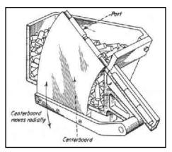
A centerboard selector is similar to reciprocating feed. The centerboard top can be milled to various section shapes to pick up moderately complex parts. I works best, however, with cylinders that are too long to be led with the reciprocating hopper. The feed can be continuos or as required.
