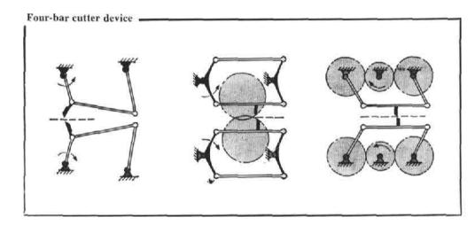
These 3 four-bar cutters provide a stable, strong, cutting action by coupling two sets of links to chain four-bar arrangements.
