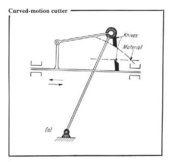
The material is cut while in motion by the reciprocating action of the horizontal bar. As the bar with the bottom knife moves to the right, the top knife will arc downward to perform the cutting operation.
