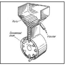
A long-cylinder feeder is a variation of the first two hoppers. If the cylinders have similar ends, the parts can be fed without proposition, thus assisting automatic assembly. A cylinder with differently shaped ends requires extra machinery to orientated the part before it can be assembled.
