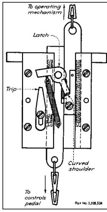
**Fig. 1** A repetition of the machine cycle is prevented if a pedal remains depressed. The latch carried by the left slide pushes the right slide downward with a curved shoulder until the latch is disengaged by trip member.
