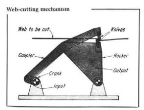
This four-bar linkage with an extended coupler can cut a web on the run at high speeds. The fourbar linkage shown is dimensioned to give the knife a velocity during the cutting operation that is equal to the linear velocity of the web.
