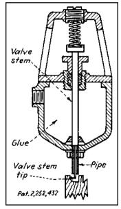
Fig. 14 A shoulder on a valve stem in a glue chamber retains glue until pressure on the tip opens the bottom valve.
