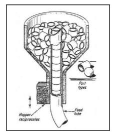
A **reciprocating feed** for spheres or short cyclinders is one of the simplest feed mehanisms. Either the hopper or the tube reciprocates. The hopper must be kept topped-up with parts unless the tube can be adjusted to the parts level.
