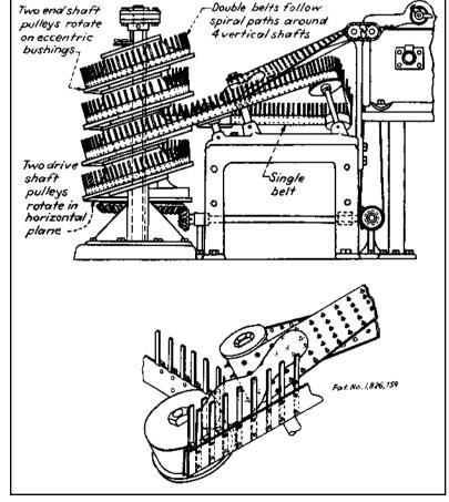
A double belt sandwiches shoe soles during their cycle around a spiral system and then separates to discharge the soles.
