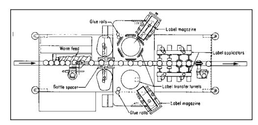
The flow of containers through this labeler is shown by the top-view drawing of the machine. Bottle spacers ensure that containers remain 7% in. apart on the conveyor. Dual label-transfer turrets allow for the simultaneous application of front and back labels.
