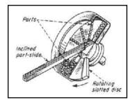
A rotary screw-feed handles screws, headed pings, shouldered shafts, and similar parts in most hopper feeds, random selection of chance-oriented parts calls for additional machinery if the parts must be fed in only one specific position. Here, however, all screws are fed in the same orientation) except for slot position) without separate machinery.
