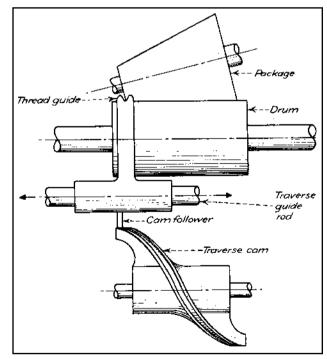
**Fig. 7** A traverse cam imparts reciprocating motion to a cam follower that drives thread guides on traverse guide rods. The package is friction driven from the drum. Yarn is drawn from the supply source through a thread guide and transferred to the drum-driven package. The speed of this mechanism is determined by the weight of its reciprocating parts.
